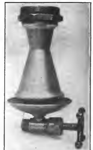
Fig. 12—The floatless carbureter of the Anzani motors
